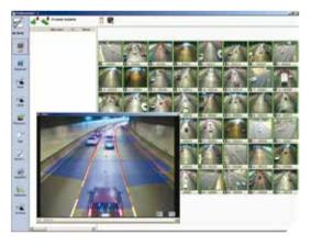
The latest Citilog Automatic Incident Detection System was installed, along with AXIS P7216 Video Encoders to take analogue data and change it into multiple video streams for the purpose of analytics.
